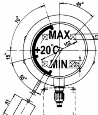
\* The oil level should be approximately at the level of 20 C at 20 C oil temperature.
